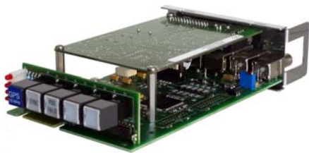
GPS 10MHz H1 module front view
